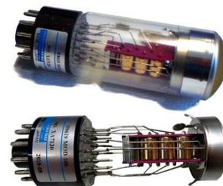
As analyser components, PMTs are considered relatively robust. Their ability to enable accurate identification and measurement of the elements for which they are configured has been proven over many years. In terms of performance, they are noted for high gain, low noise, and good speed of measurement. Their excellent trace element detection capability is aided by their markedly high dynamic range.
